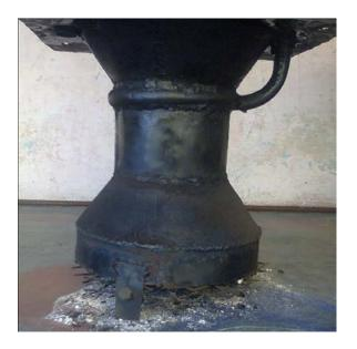
Lower diameter is of 250mm with 80mm height. A cylinder of 150mm diameter and 100mm height is welded at the top of divergent section. A circular pipe of <sup>3</sup>/<sub>4</sub> inch (approximately 20mm) diameter is Made round with internal diameter 220mm and external diameter 260mm. 8 hole of 6cm diameter is drilled.
