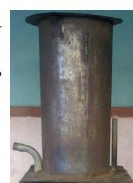
purpose of is to store biomass continuous reaction chamber. It mounted the reactor gasifier. The fuel storage hopper is made up of 2mm thick mild steel. The diameter and height of fuel hopper is chosen to be 250mm and 550mm respectively. Round shaped hopper has been chosen to prevent the problem of biomass being stuck.
